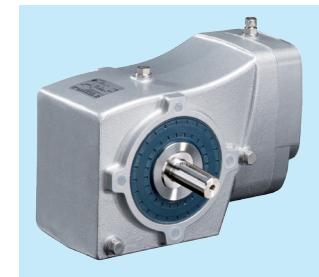
With the SK93072.1 - SK93772.1 version it is possible to machine the horizontal and vertical surfaces of the housing in order to achieve the axis heights of the SK92072.1 - SK92772.1 series. It is also possible to position threaded holes in the same location as the foot mounting holes of the SK92072.1 - SK92772.1 series, so that this housing can be optionally converted to a foot mounted housing with **B14 attachment**. On request, this version can also be implemented by reworking.
